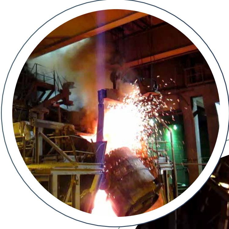
Metal Pouring into the MOR – Before
