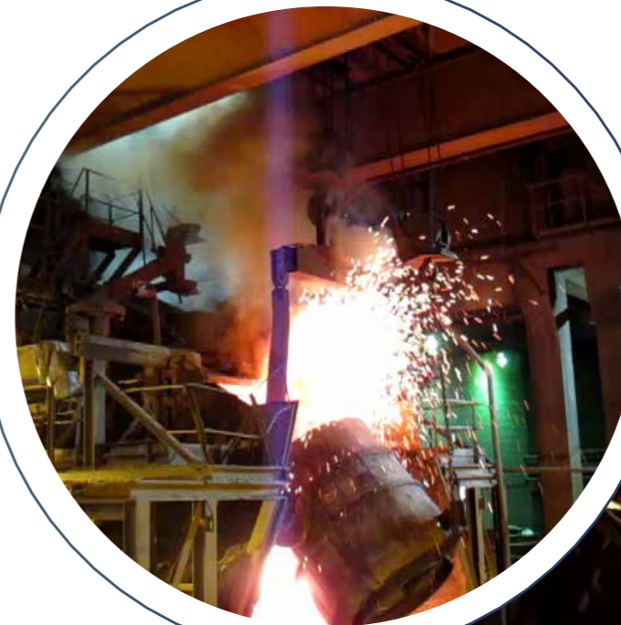
Metal Pouring into the MOR – Before
