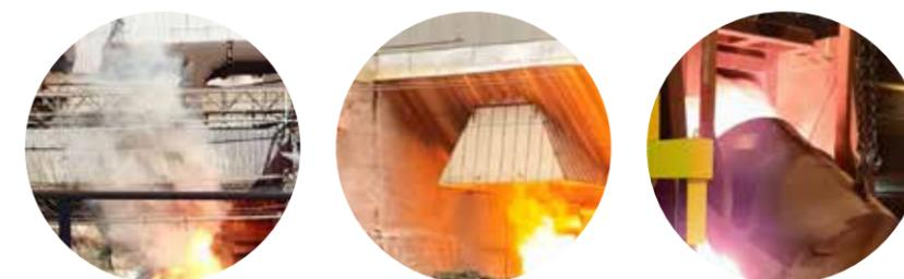
*Casting slag before installing the exhaust system (left) and effective extraction of smoke discharge after installation of the system (centre) and from the pouring point (right)*
